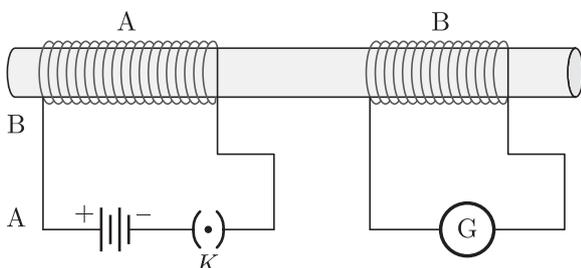
Connect coil A with a battery and coil B with a galvanometer. When the key is plugged in, the current passes through coil A and current is induced in coil B. When the key is disconnected, the galvanometer will again show deflection due to induction of current but in opposite direction. This induction is due to the variation of current in the first coil.
