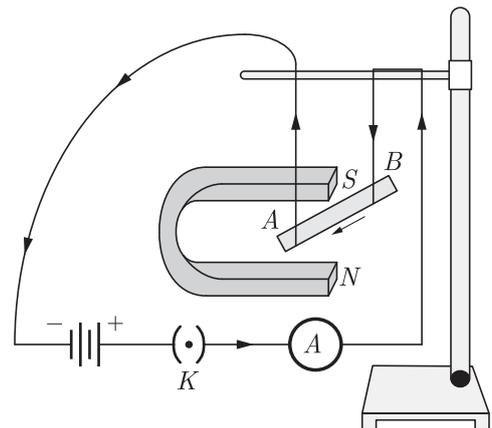
3. Now connect the rod AB in series with a battery, a key and a rheostat and allow the current to pass through the rod from B to A. You will find that the rod gets displaced instantaneously towards the left.
