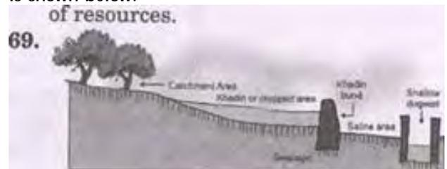
The structure of a traditional water harvesting system. In largely level terrain, water harvesting structures are generally crescent shaped earthen embankments or low , straight, concrete and rubble, check dams, built across a seasonally flooded gullies. Monsoon rains fill the ponds behind structures. Only the largest structure hold the water year round. Most of them dry up six months or less after the monsoon.
