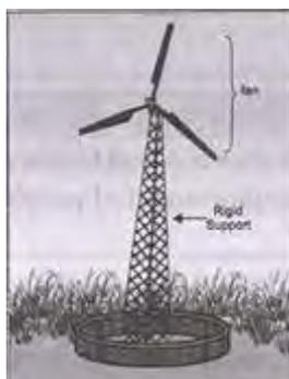
The energy of wind mill was harnessed in the past in doing mechanical work e.g., in water lifting pump, the rotatory motion of wind mill is utilised to lift water from the well.
