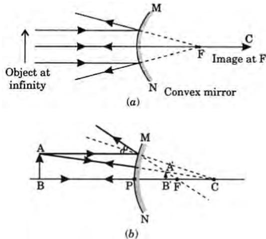
Convex mirrors are used in automobiles as a rear view mirror because of wider field of view and formation of erect image.
