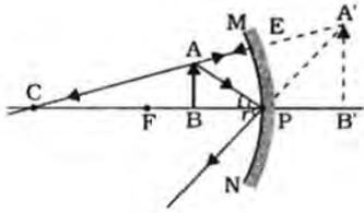
Real and magnified image will be formed if the object is placed in between  $2F(C)$  and  $F$  in front of a concave mirror.
