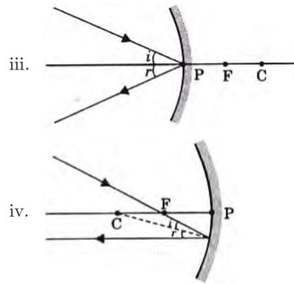
76. (a) Draw a ray diagram in each of the following cases to show the position and nature of the image formed when object is placed:
