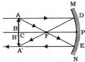
37. Draw a ray diagram for the image formed by a concave mirror when the object is placed beyond its centre of curvature.
