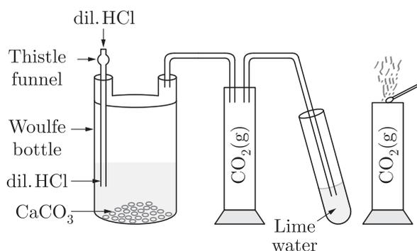
Reaction of calcium carbonate with dilute hydrochloric acid to liberate carbon dioxide gas which turns lime water milky and extinguishes burning matchstick
